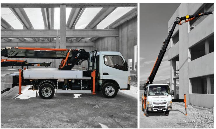
2,41 m, 1,88 m width and 6,17 m length. The hydraulic boom can reach up until 21.60 m height and can lift 4.000 kg at minimum outreach.
