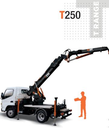
2,17 m, 1,72 m width and 4,77 m length. The hydraulic boom can reach up until 16,50 m height and can lift 2.500 kg at minimum outreach.
